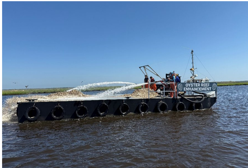
Loose broadcasting of recycled shell using a barge and water cannon. Credit: NJDEP
