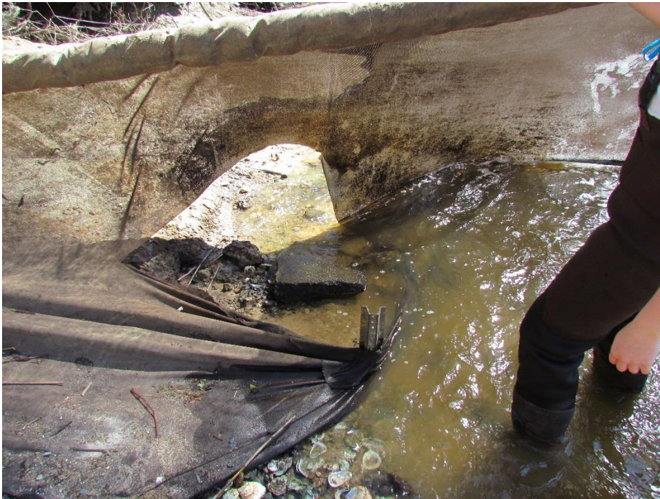
Figure 5. Damage to fyke net due to high flows at the sampling site.
