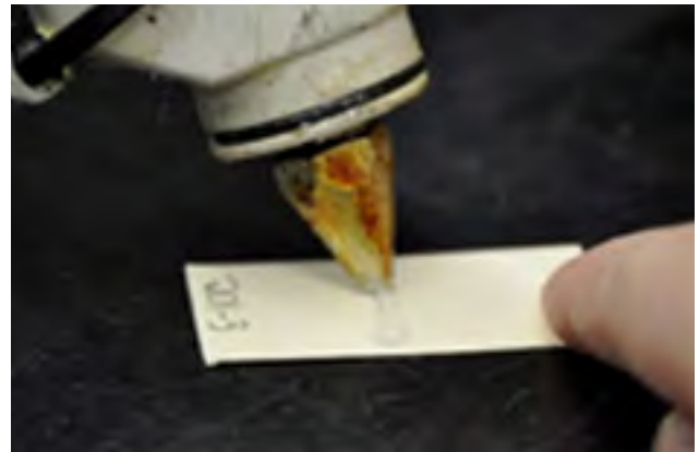
Figure 3.28 Hot-melt glue applied to small strip of cardstock ready to receive whole otolith for sectioning using the multi-blade sectioning technique.
