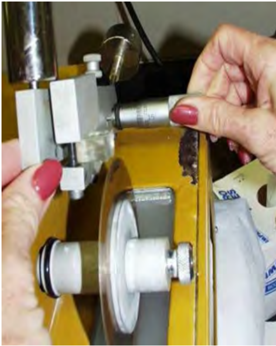
Figure 3.25 Alignment of the block to the blade is made by adjusting the micrometer.
