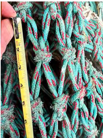
Photo #2 Non compliant mesh in the lengthener
