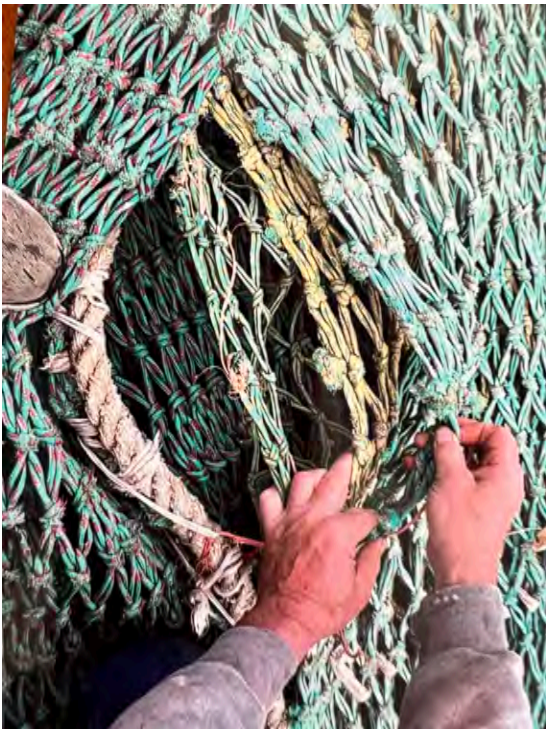
Photo #4 Chaffing gear on bottom of lengthener
