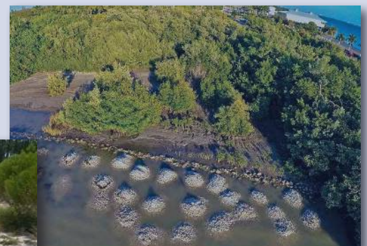
Punta Rassa, Florida after living shoreline installation (above). A living shoreline constructed in Panama City, Florida using plants and oyster shell (left). Photo credit: www.floridalivingshorelines.com .
