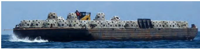
Existing “DRH” offshore artificial reef site; 130 pallet balls deployed. Photo Credit: January Murray, Georgia Department of Natural Resources (GA DNR)
