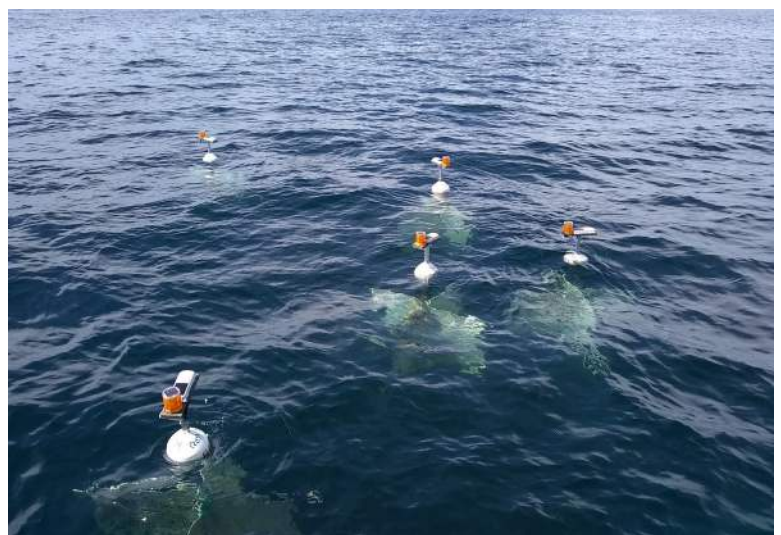
Ocean drifters floating after being released from R/V Endeavor. Drifters include a GPS device, solar powered light, and contact information. Image credit: Wells National Estuarine Research Reserve.
