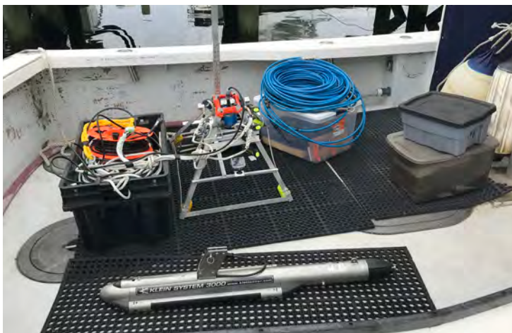
Side-scan sonar and photo/video survey equipment used for site selection (left). Photo credit: MA DMF. Divers collecting data along a transect (right). Photo credit: MA DMF.
