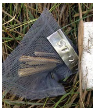
Figure 4. Example of litterbag used to measure decomposition. Photo by S. Buckley.
