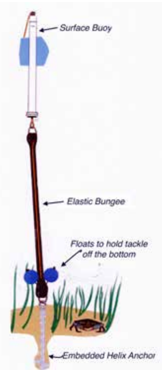
Hazelett Conservation Mooring System
