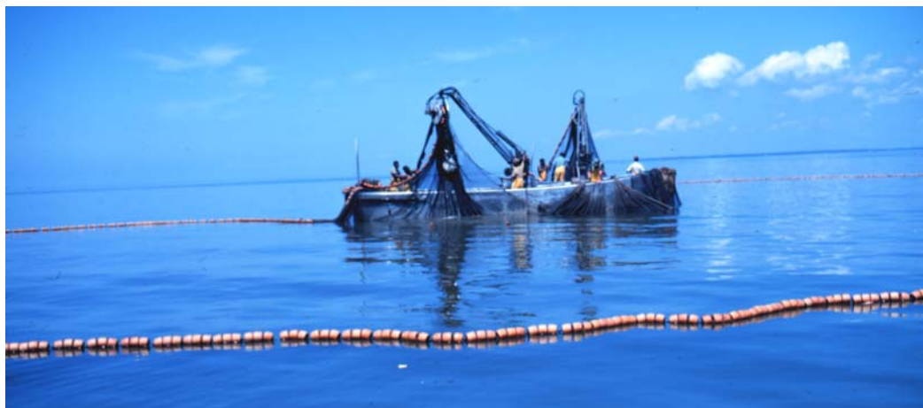
Menhaden purse seine vessels and net (Photo courtesy of Robert K. Brigham, NOAA, Dept. of Commerce)
