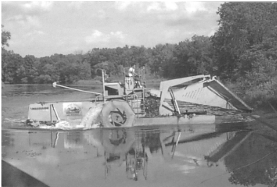
Figure 1. Mechanical aquatic weed harvester used in deep water areas of the Hockanum River, CT to help eliminate water chestnut, an invasive, non-native plant. Courtesy of the Connecticut Department of Environmental Protection's Office of Long Island Sound Programs.
