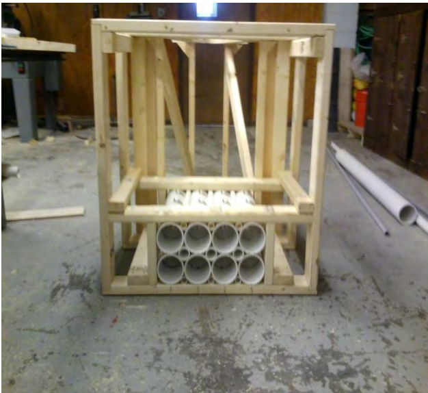
Figure 11. Top: Front view of the counter head that consists of eight four inch PVC tubes fitted with three stainless steel clamps, acting as sensors that measure water conductivity. Bottom left: View of fish counter head during construction. Bottom right: View of in-stream weir and fish counter.
