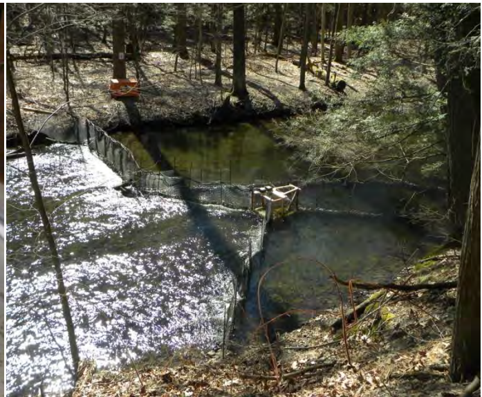
Figure 11. Top: Front view of the counter head that consists of eight four inch PVC tubes fitted with three stainless steel clamps, acting as sensors that measure water conductivity. Bottom left: View of fish counter head during construction. Bottom right: View of in-stream weir and fish counter.
