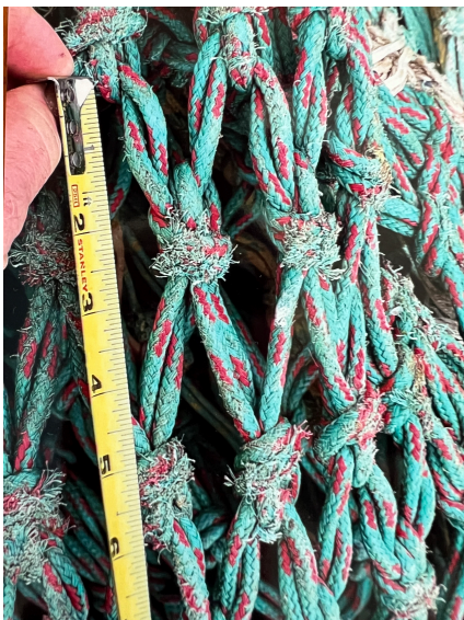
Photo #2 Non compliant mesh in the lengthener
