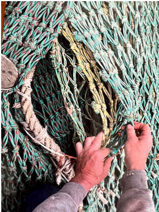
Photo #4 Chaffing gear on bottom of lengthener
