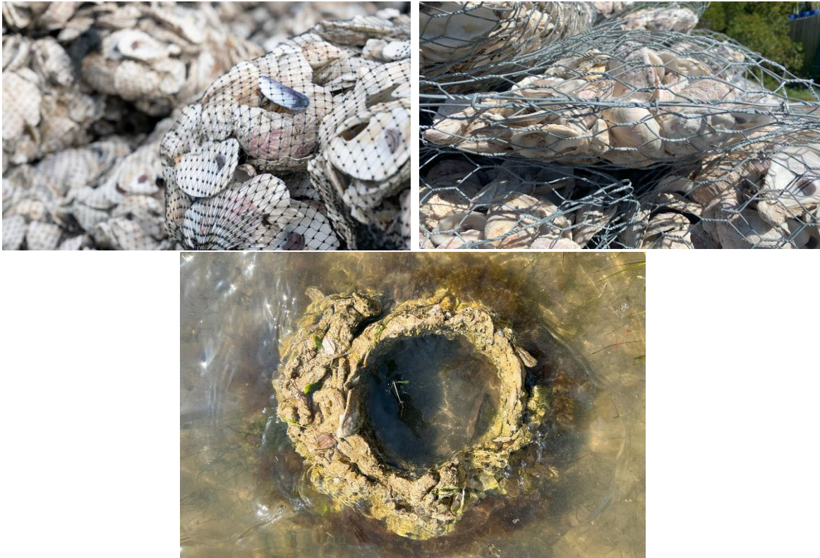
Top left: Naltex mesh oyster bags. Top right: double-galvanized steel “soft gabions”. Bottom: jute and cement volcano.
