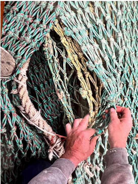
Photo #4 Chaffing gear on bottom of lengthener
