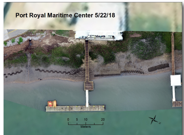
UAV imagery of the SCDNR deployment of different reef substrates. Photo credit: SCDNR.
