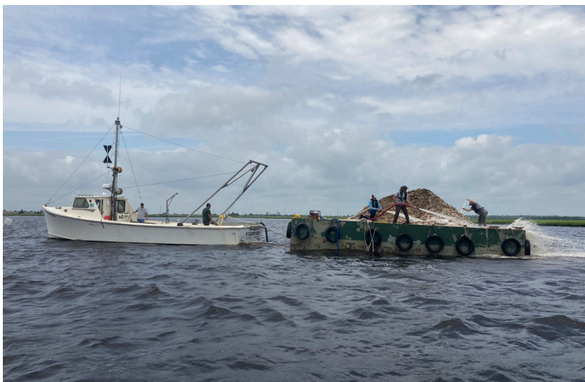
Using water cannons to deploy shell onto reefs. Image credit: NJDEP MFA.
